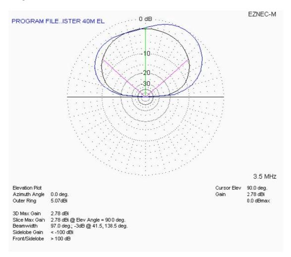
The full loop on 80M and 40M. Here is a comparison between the full 80m loop vs. the 40m delta loop, both transmitting on the 40m band i.e. 7MHz.
