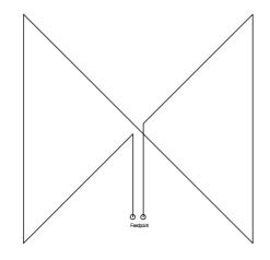
The wire length is a full wave length on 80M. A full wave loop has two current maxima, which means that maximum radiation takes place at two places on the loop,
